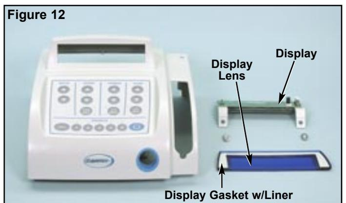
Then, remove the other plastic liner backing from the face of the Gasket and press Display Lens onto the front of the display opening on the top cover. (**NOTE:** Ensure that the inside face of Lens is clean and free of dust before applying to top cover.)
