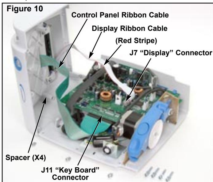
12. Note orientation of Control Panel flex cable with "Key Board" connector 'J11' on PCB Assembly (see Fig. 10). Detach flex cable from connector 'J11'.
