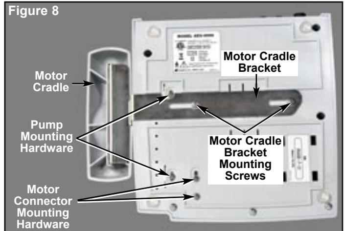
7. Slide Motor Harness Assembly (PN: 875103) and Bracket (PN: 461814) backwards in slotted hole so that Motor Connector disengages from blue bezel in cover. Lightly tighten mounting screw to secure Harness/Bracket in place.
