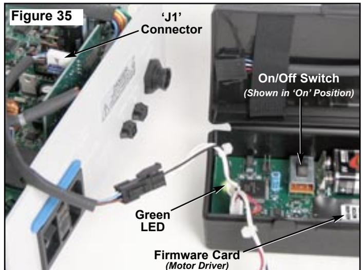
9. The Green & Red LED's on the Programmer will operate in the following sequence when programming is successful: **IMPORTANT:** The Red LED will remain On in the event of improper programming.
