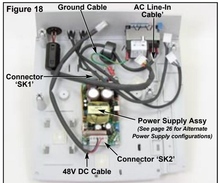
23. Locate and cut the Cable Tie (PN: 510137) that attaches the AC Line-In Cable (PN: 875106) to the Chassis. Detach AC Line-In Cable and Ground Cable Wire (PN: 875085) connectors from wire terminals on Power Inlet Assembly (PN: 840086) (see Fig. 19). Make note of wire/terminal orientation and cable loops through ferrite before removing Cables. (**NOTE:** During reassembly, ensure that the black wire of AC Line-In Cable is attached to the outside terminal on Power Inlet Assembly.)
