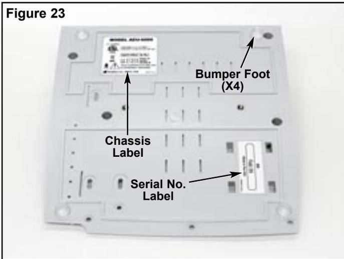
29. Turn Chassis base (PN: 461728) over to expose four rubber Bumper Feet (PN: 850069) on bottom side (see Fig. 23). Replace as necessary.
