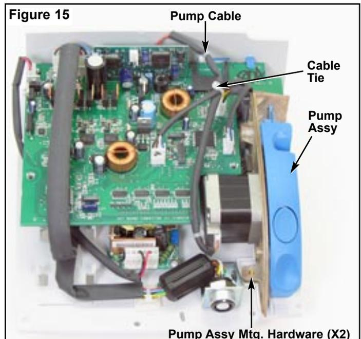
19. Disconnect all cable and wire connectors from PCB Assembly (PN: 330559). Make note of each cable's routing and connector/pin orientation before disconnecting from PCB (see Fig. 15). Cut and remove cable ties as necessary. Pinch the snaps
